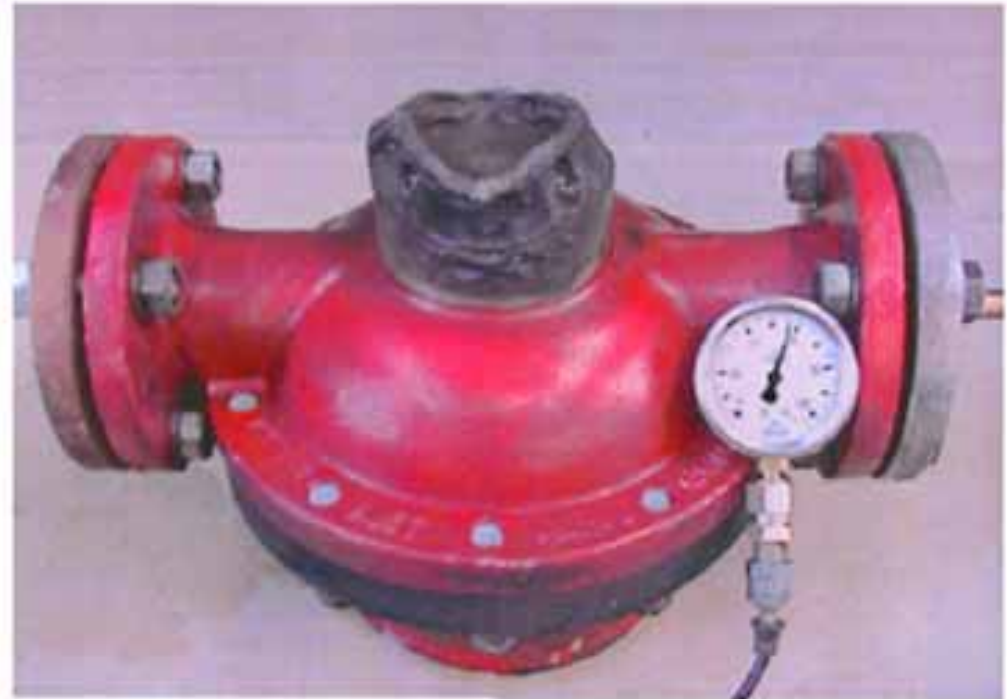
Figure 7: Sensor housing of CONTOIL® OIL flow meter of the nominal size of 50 mm during the pressure test
